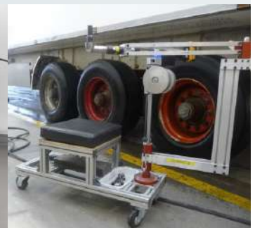
Mobile workstation for tightening under truck body (torque 75 Nm) DOC.40662
