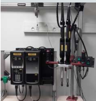
Synchronised double-spindle (center distance 55 mm) DOC.40991
