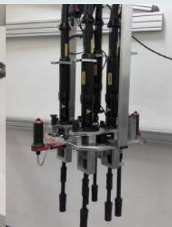
6 spindles screw head (variable center distances, tightening torque 100 Nm) DOC.40620
