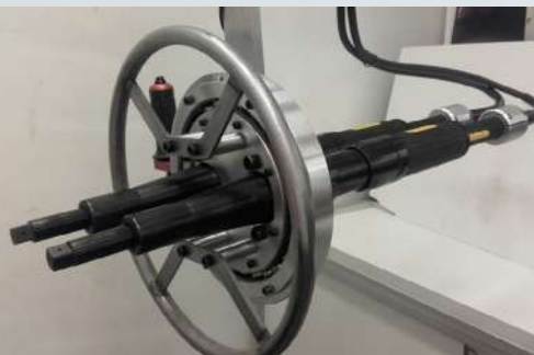
Double-spindle for wheel tightening (torque 105 Nm, center distance 100 mm) DOC.40453
