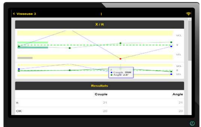
Visualisation of the last tightening and storage of results for analysis
