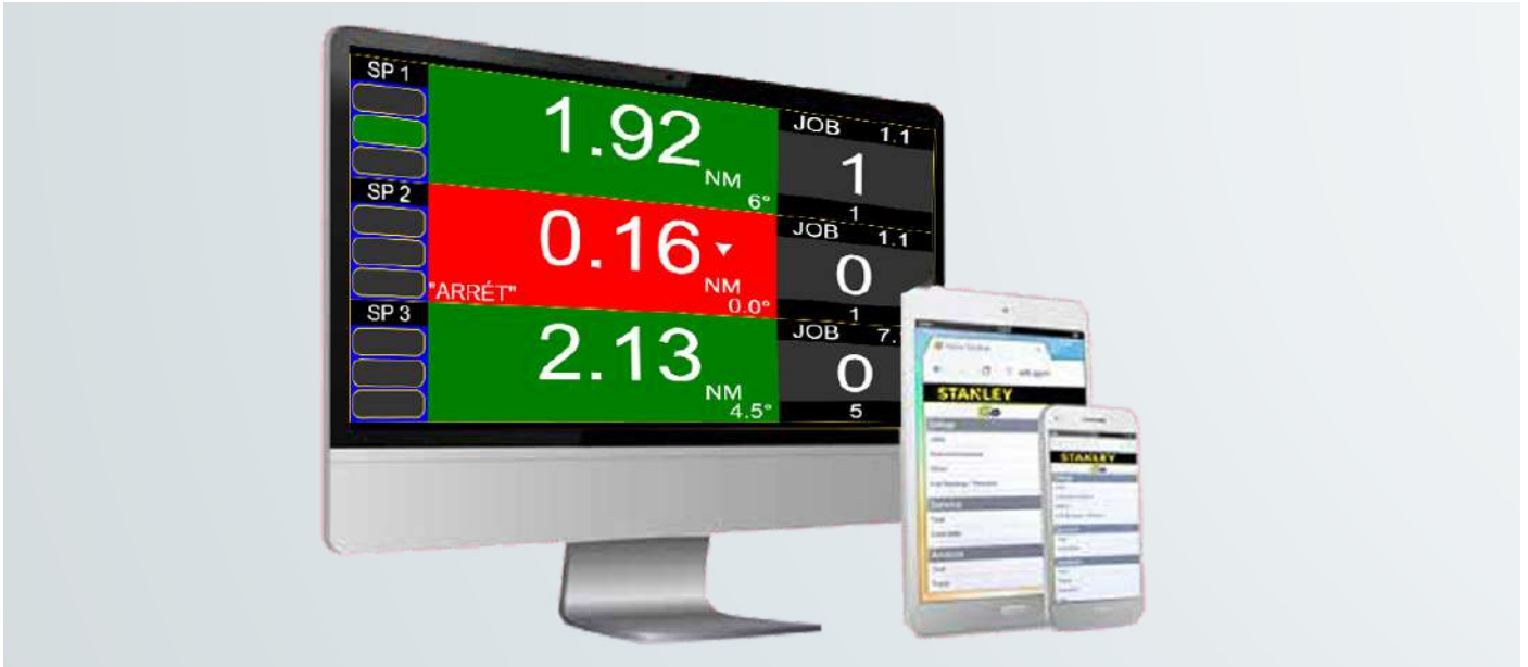
Visualisation of the last tightening and storage of results for analysis
