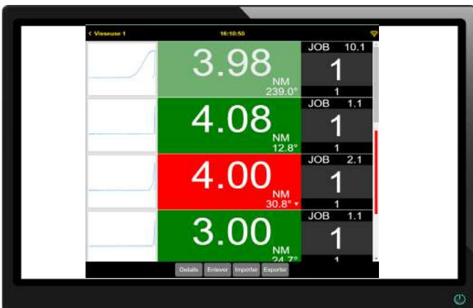
Visualisation of the last tightening and storage of results for analysis
